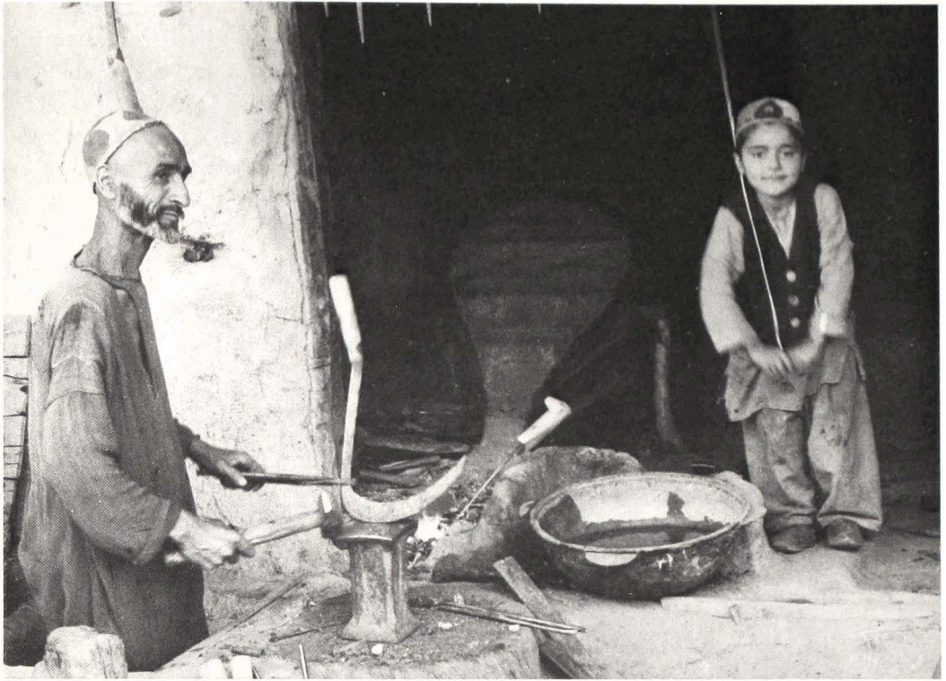
Tashqurghan: Blacksmith ( ustad ) working on a sickle outside his workshop on Black/Wood Street. A chagird assists him with the bellows.
